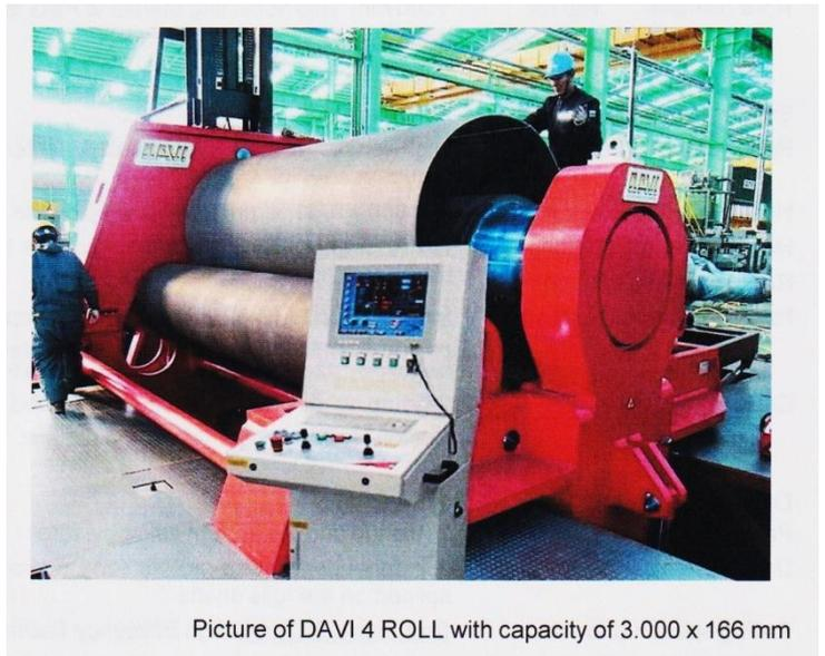
Picture of DAVI 4 ROLL with capacity of 3.000 x 166 mm
